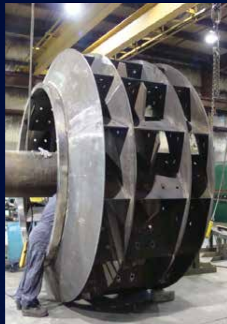
PELLETIZING PLANT - BAHRAIN 130" dia. Backward Inclined, DWDI ASTM A514 Gr. S High Strength Steel Wear Protection: Chromium Carbide
